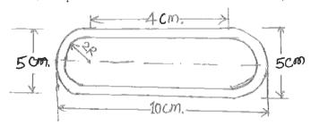
Calculate the weight of 50 metres of a steel chain, one link of which is shown fig. Link is made from 1 cm diameter rod. The weight of rod material is 6.6 gm/cm length.
