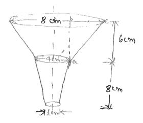
Estimate the cost of metal sheet for preparing a funnel as shown in fig. Assume the wastage of metal as 10% and cost of the sheet as ₹ 20/m<sup>2</sup>.
