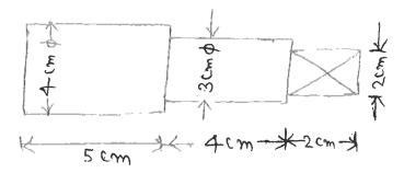
200 pieces of a component as shown in fig. are to be drop forged from a 4 cm dia stock bar. Calculate the cost of manufacturer, if:
