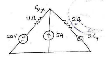
Determine the voltage across the terminals AB in the circuit shown in fig.
