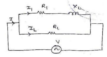
In the circuit shown in fig., the current is at its maximum value with capacitor value  $C = 20 \,\mu\text{F}$ and 0.707 times its maximum value with  $\,C=30\,\mu F$  . Find the value of Q at w = 500 rad/sec and circuit constants.
