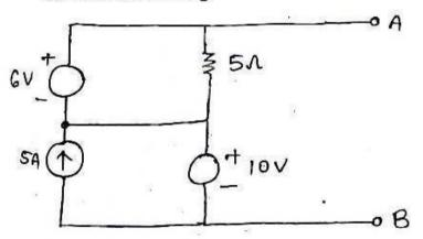
Calculate the current I shown in fig. using Millman's theorem.
